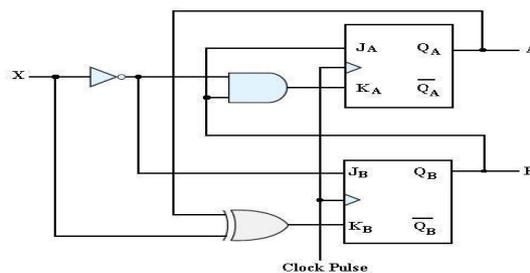
10. Design a clocked synchronous sequential logic circuit for the following state diagram.
