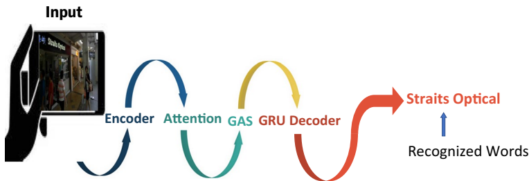
Fig. 15 Sequence to sequence domain adaptation framework for text recognition (Zhang et al. 2019)
