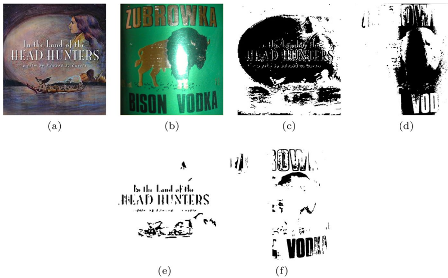
Fig. 6 Progress in pre-processing of scene text image. The source image a represents a Hollywood movie poster, and b is taken from a bottle cover. The output of Otsu's binarization technique (Otsu 1979) are shown in (c, d) and the binarized images generated by an auto-encoder-based approach (Calvo-Zaragoza and Gallego 2019) is presented in (e, f) for the images shown in (a, b) , respectively
